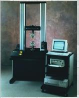
**Dynamic - Higher rates** of speed, cycling, frequencies; servohydraulic.
